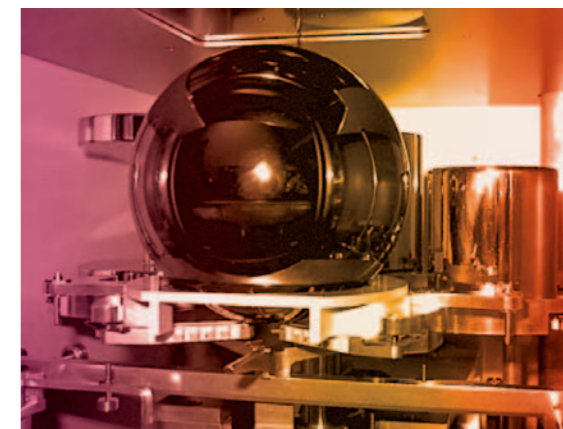
Photograph of the 1kg silicon sphere set in the vacuum mass comparator S Mizushima, M Ueki and K Fujii Metrologia 41 S68–S74.
