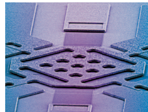
Tuneable RF-MEMS capacitor (courtesy of Philips). M G D Geers, W A M Brekelmans and C J Bayley 2007 Modelling and Simulation in Materials Science and Engineering 15 S133–S145.
